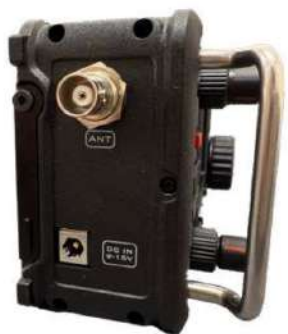
Figure 1 — The Xiegu X6200 left side, showing the RF and dc interfaces.
