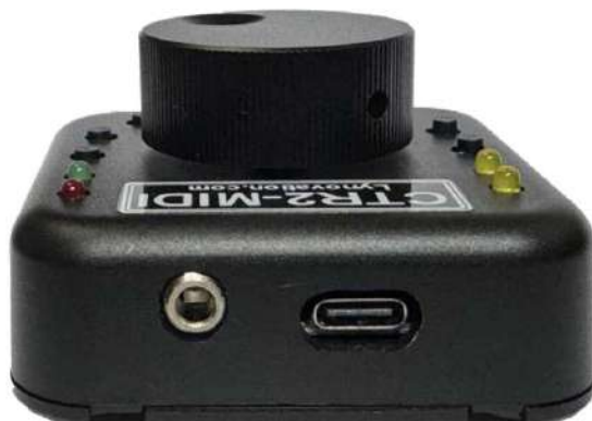
Figure 7 — The CTR2-MIDI rear panel.
