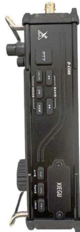
Figure 3 — The Xiegu X6200 top side, showing the mode, band, ATU, and expansion port.
