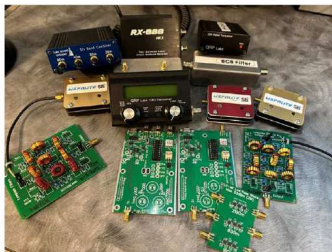
Figure 2 — Some of the available WSPR transmitters, transceivers, and filters.
